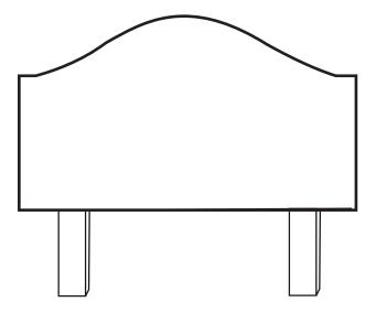
Attach 2 x legs (B) to 1 x bedhead (A) as shown and secure with 6 x washers (C) and 6 x bolts (D). Tighten with an Allen Key (E).
